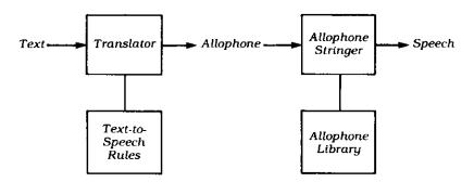
When you input text to be spoken, the module first translates the English text into its allophonic equivalent, using the speech rules programmed into the module. The rules also include symbols for sentence contouring. Next, the allophone strings, which may include pitch modifiers, are converted to Linear Predictive Coding (LPC) strings. The LPC strings are then processed through the Speech Synthesizer and spoken.
