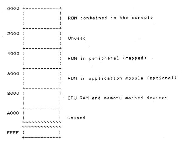
The peripheral ROM is mapped in to memory by selection through the CRU. The peripheral devices each have a unique CRU address. An access to that address maps the ROM for that device into the memory map. This addressing is further described in "Home Computer System Memory, CRU, and Interrupt Mapping Specification."
