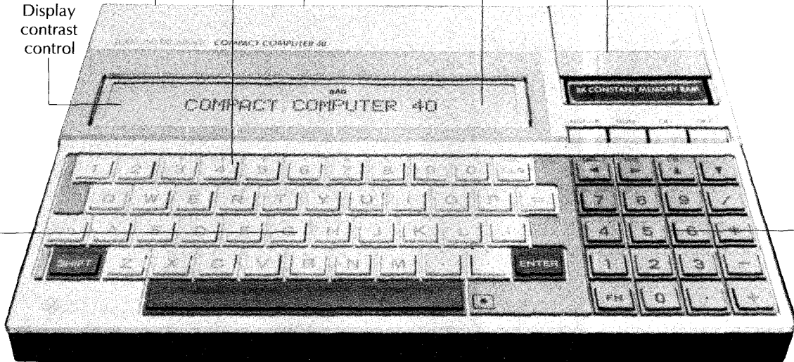
Fig. 1-2 The Texas Instruments CC-40 standard QWERTY keyboard and numeric keypad with cursor control keys make calculations and text and data entry quick and easy.
